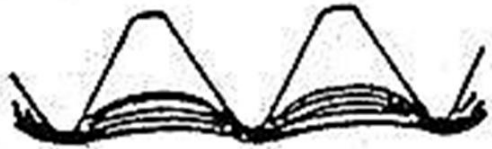
FIGURE 1 – ROLLED THREAD FLOW LINES
